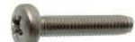
62222 PAN HEAD THREAD ROLLING SCREW CROSS RECESS POZIDRIVE DIN 7500 CZ - STAINLESS STEEL A2
