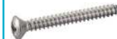
64411 RAISED COUNTERSUNK HEAD TAPPING SCREW FORM C CROSS RECESS POZIDRIVE ISO 7051 DIN 7983 - STAINLESS STEEL A4
