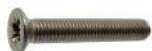
30101 COUNTERSUNK FLAT HEAD MACHINE SCREW CROSS RECESS POZIDRIVE DIN 965 4.8 CLASS - ZINC PLATED
