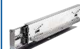
B3-07 Slides with brackets for on-board equipments - Max 150 - 180 kg per pair - Stroke +100% - Zinc Plated Steel
