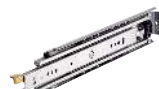
B3-090 Slides 2 positions Stop - Max 154 - 227 kg per pair - Stroke 100% - Zinc Plated Steel
