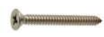
64408 RAISED COUNTERSUNK TAPPING SCREW FORM C CROSS RECESS POZIDRIVE ISO 7050 DIN 7982 - STAINLESS STEEL A4
