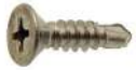
62428 COUNTERSUNK HEAD SELF DRILLING SCREW CROSS RECESS "PHILLIPS" DIN 7504 0 H - STAINLESS STEEL A2
