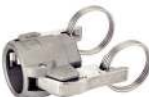
5528 BSP threaded female coupler with safety locking cams - NBR gasket - Stainless steel 316
