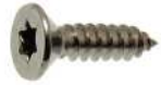
62410 RAISED COUNTERSUNK HEAD TAPPING SCREW FORM C CROSS RECESS SIX LOBE DIN 7982 - STAINLESS STEEL A2
