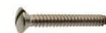
62404 SLOTTED COUNTERSUNK RAISED HEAD TAPPING SCREW FORM C DIN 7973 - STAINLESS STEEL A2
